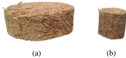
Figure 11 Acoustic absorption test specimens (ISO 10534-2) (a) Specimen with a diameter of 9.8 cm (b) Specimen with a diameter of 2.8 cm
