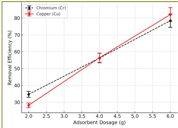
Figure 2. Removal efficiency for various adsorbent dosage
