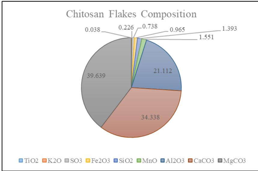
Figure 1. XRF analysis of chitosan flakes composition
