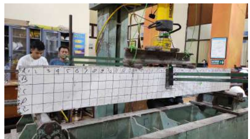
Fig. 5. Testing process of the splice beam.
