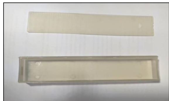
Figure 10 The actual specimen is injection molded from parameters obtained from the experimental design; Taguchi and Statistical Analysis Program of PP-L Plastic.
