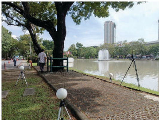
Figure 2 Scanner (TLS) and reference spheres positions in the field.
