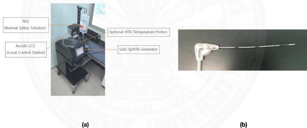
Fig. 1.6 the equipments of the MWA system at Office of Advanced Science and Technology, Thammasat University; (a) the microwave generator (Acculis, AngioDynamics, 60-140 W, 2.45 GHz), (b) microwave antenna (Accu2i PMTA Applicator)
