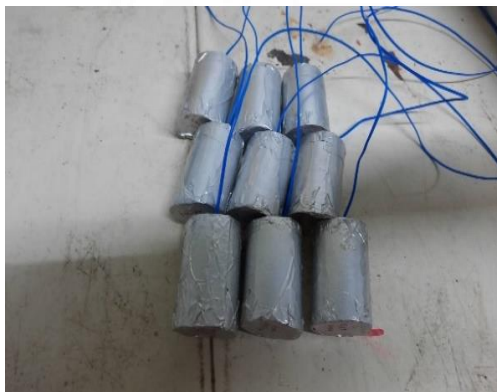
Figure 5.1c Firmly wrapped specimen with aluminum foil
