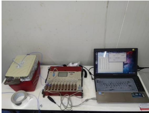
Figure 5.3 The apparatus for specific heat testing
