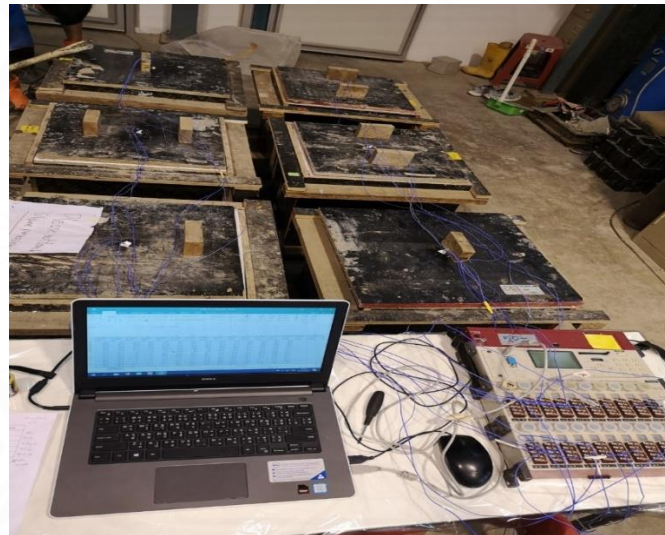
Figure 9.10 Specimens with the temperature rise history recording system
