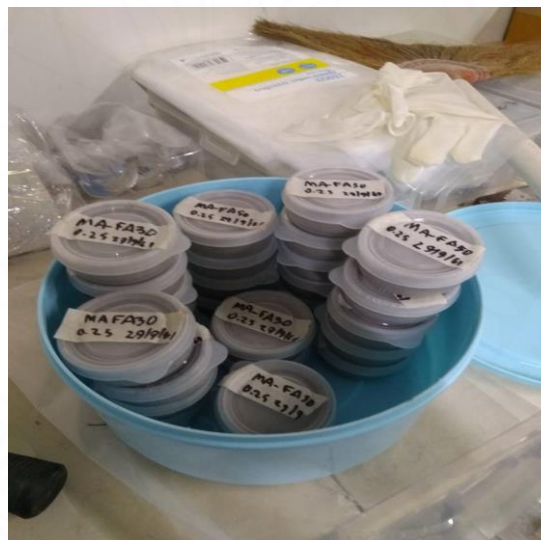
Figure 4.2 Container for keeping the free water content testing molds in the control room
