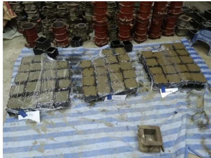
Figure 9.3 The specimen's preparation in the plastic cube covered with the plastic wrap
