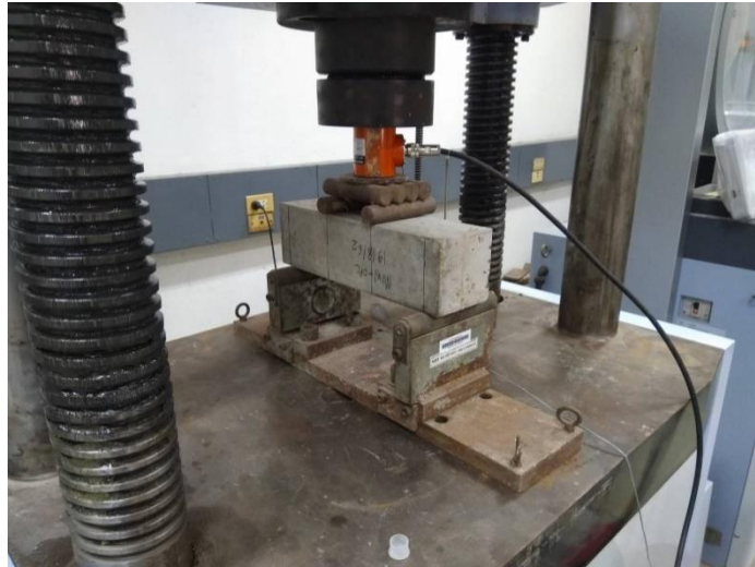
Figure 9.7 Experimental setup for tensile strain capacity testing
