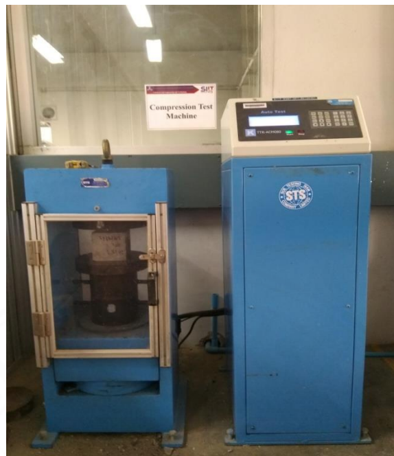
Figure 9.4 The experimental setup for the compressive strength testing
