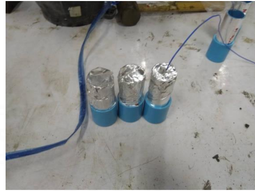
Figure 5.1b Aluminum foil covered after finished casting specimen
