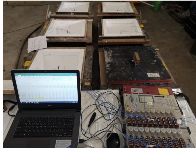
Figure 9.9 Experimental setup for the semi-adiabatic temperature rise testing
