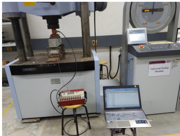
Figure 9.6 Apparatus for tensile strain capacity testing
