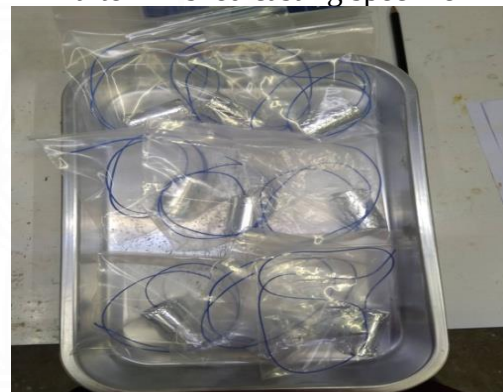
Figure 5.1d Zip-lock plastic used for covering specimens until the testing age
