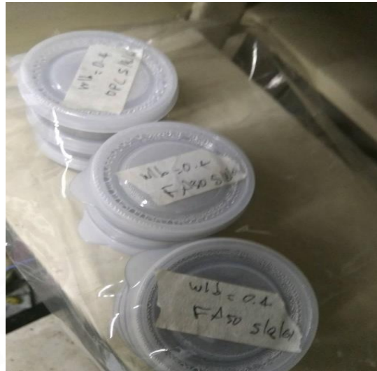
Figure 4.1 Plastic molds completely sealed for the free water content specimen
