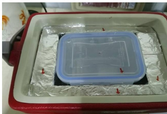
Figure 5.2 The insulated container for specific heat testing
