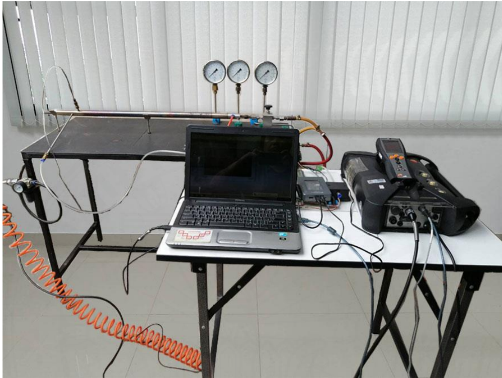
Figure 3.7 Testing combustor and data acquisition for optimal control design.
