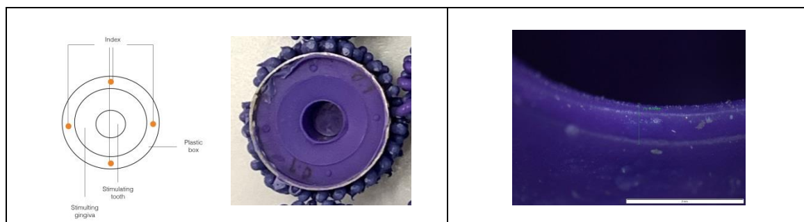
Figures 3 3a (Left) The extension of the impressions that penetrated the stimulated sulcus ; 3b (Right) Penetration of the impression material into the gingival sulcus obtained from Image-Pro Plus image analysis software (Media Cybernetics, Inc., USA)
