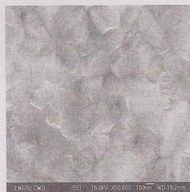
Fig. 2 Typical SEM micrograph of rutile TiO 2 thin films at temperature 700°C
