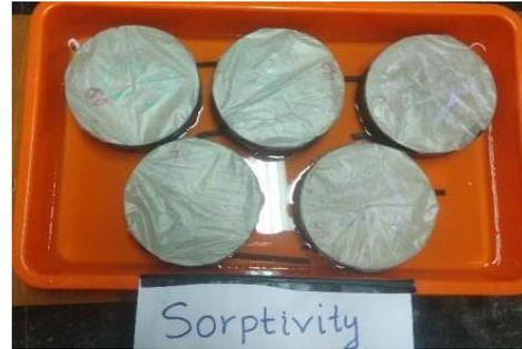
Figure 2. Test setup for sorptivity.
