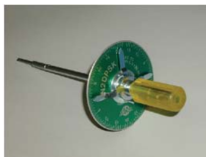
Figure 28 Torque screw driver (N2DPSK, Nakamura MFG Co. Ltd) used to record the placement torque of the mini-screw. This device has a round dial gauge with a pointer to read the peak value.
