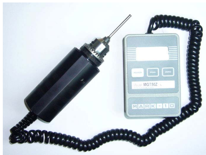
Figure 32 Digital torque gauge with a chuck grips the hand driver tip.
