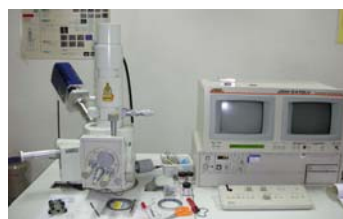
Figure 25 EDS-SEM: JSM-5410LV JEOL LTD, Tokyo, Japan
