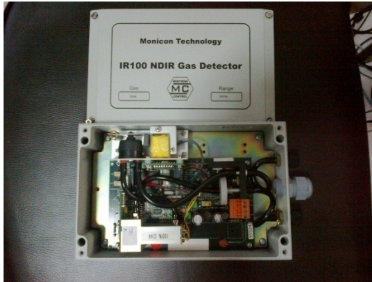
Fig. 2.10 Monicon IR100 NDIR Methane Sensor
