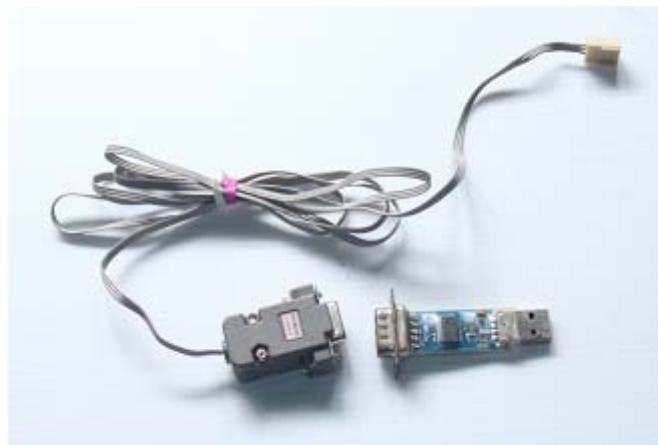
Fig 3.29 UCON-232s USB to RS232 Converter and ET-RS232 9 PIN F
