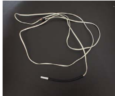
Fig 3.12 10k \Omega type thermistor
