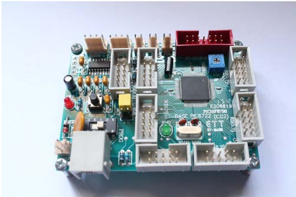
Fig 3.21 PIC18F8722 Microcontroller with programming board
