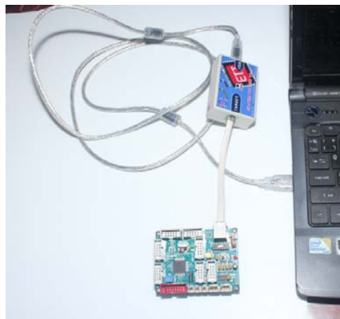
Fig 3.24 Connect microcontroller to computer using ET-PGM PIC USB2.0
