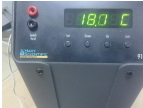
Fig 3.14: Setting standard temperature using dry well temperature calibrator
