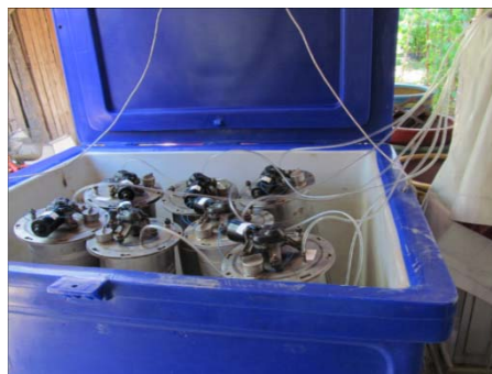
Fig. 3.4 Seven Digestion Tank in temperature control tank
