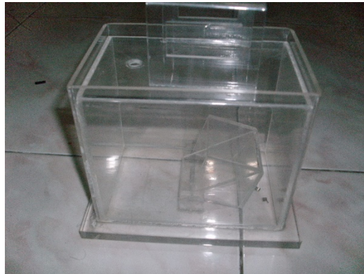
Fig 3.2 Flow meter at normal position
