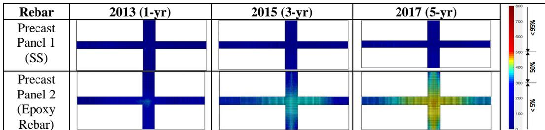
Figure 4. Newark Bay Bridge monitoring results 1 – Ag electrode.
