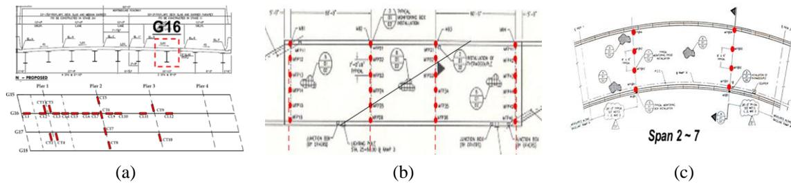
Figure 3. Sensor layout of Patcong Creek Bridge, Bridge No. 84.1 and Bridge No. 159.7A.
