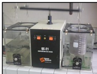
Figure 4.4 The relation times of disintegration of capsule, capsule began to disintegrate at 2 minute and completely disintegrated at 8 minute. Which BP standard defined time limit of disintegration of capsule at stomach, must not exceed 10 minute.
