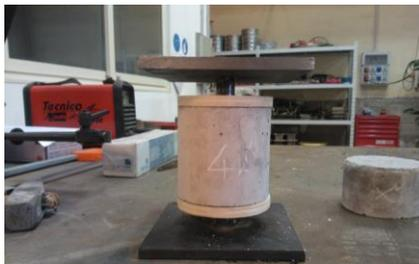
Figure 3. Punch loading system.
