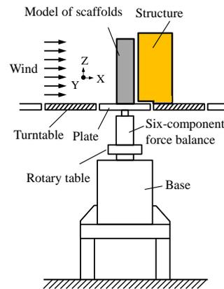
Figure 4. Six-component force balance.
