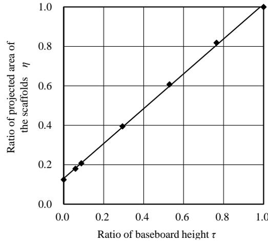
Figure 6. Relationship between the ratio of the projected area of the scaffolds and the ratio of the baseboard height.
