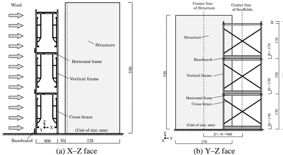
Figure 5. Scaffolds and structure used for the wind tunnel test.
