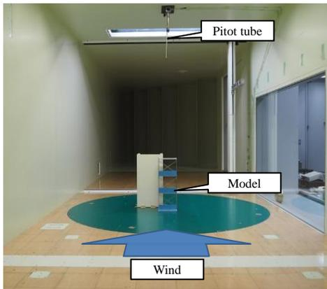
Figure 3. Wind tunnel test.
