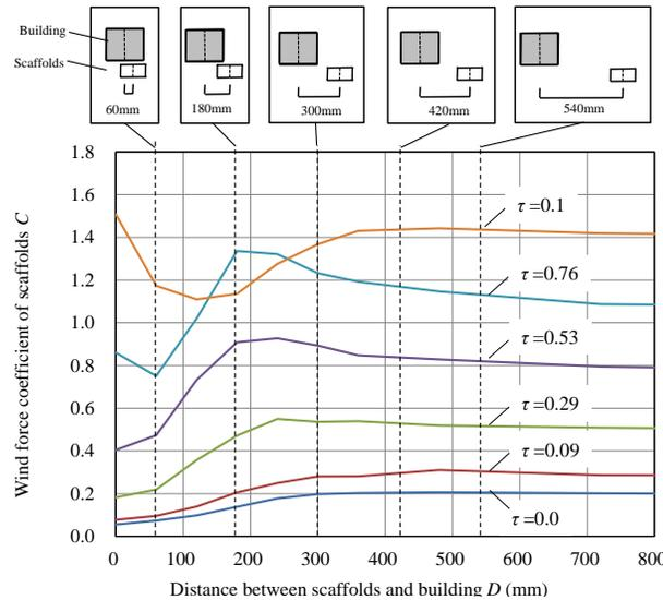
Figure 7. Relationship between the wind force coefficient and the distances between the building's center and the scaffold's center.
