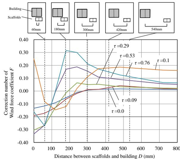
Figure 8. Relationship between the correction factor of wind force coefficient and the distances between the building's center and the scaffold's center.
