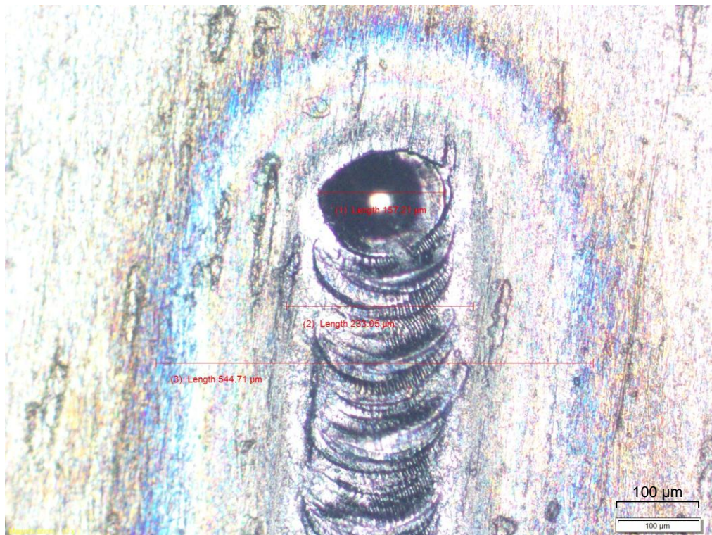
Figure 3.19 Laser ending point on Ti sheet grade 2, thickness 0.5 mm
