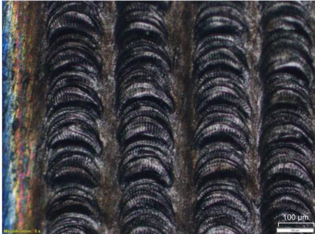
Figure 3.17 Top view of Ti at 70,000 W/cm 2 , 2 mm/s
