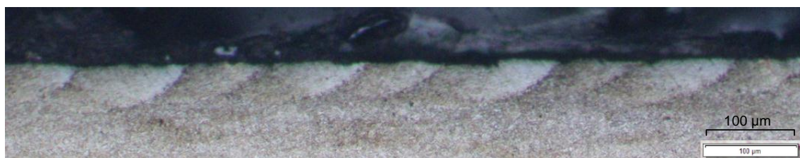
Figure 4.11 Surface of laser hardened layer with 40,000 \text{ W/cm}^2 , 2 mm/s, d = 0.1 \text{ mm}
