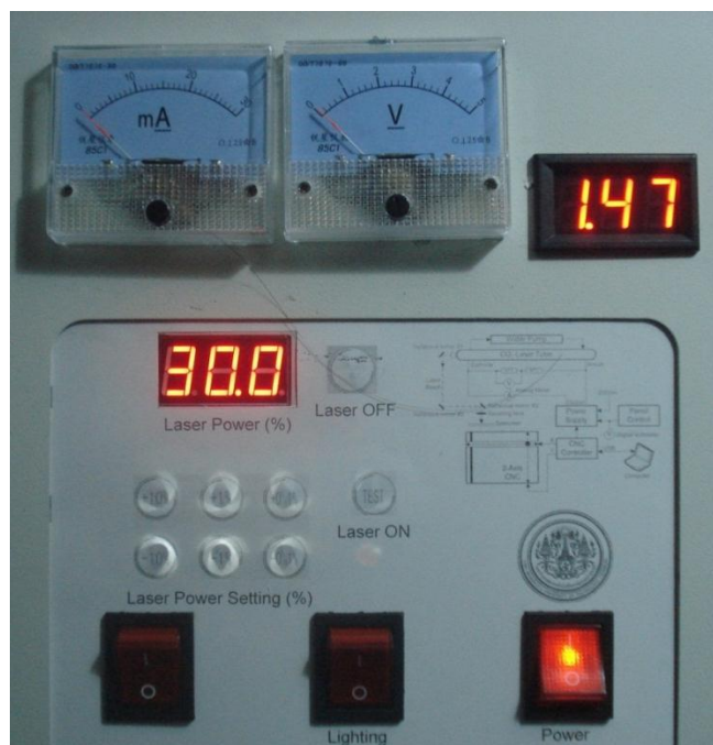
Figure 3.4 Panel control and the current and voltage measuring
