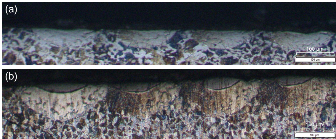
Figure 4.12 Surface of laser hardened layer of the 1045 specimen with: (a) 40,000 \text{ W/cm}^2 , 2 \text{ mm/s} , d = 0.2 \text{ mm} ; (b) 60,000 \text{ W/cm}^2 , 2 \text{ mm/s} , d = 0.2 \text{ mm}
