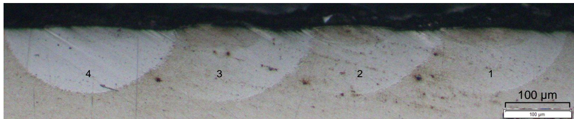
Figure 4.6 Surface of laser hardened layer with 70,000 W/cm 2 , 4 mm/s, d = 0.2 mm
