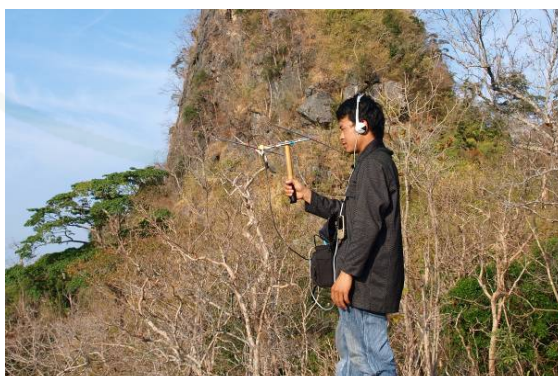
Appendix Figure 19 Signal detected using home in method in the dry season (Field assistant Mr. Jaolo).
