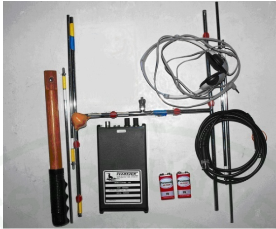
Appendix Figure 2 The receiver, two-elements Yagi antenna and telex headphone.
