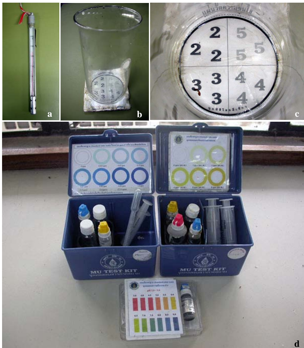
FIGURE 3.2 Materials for water quality measurement: a) pond thermometer b) and c) turbidity plate d) MU Test Kits for pH, Dissolved Oxygen (DO), and Phosphate (P)
