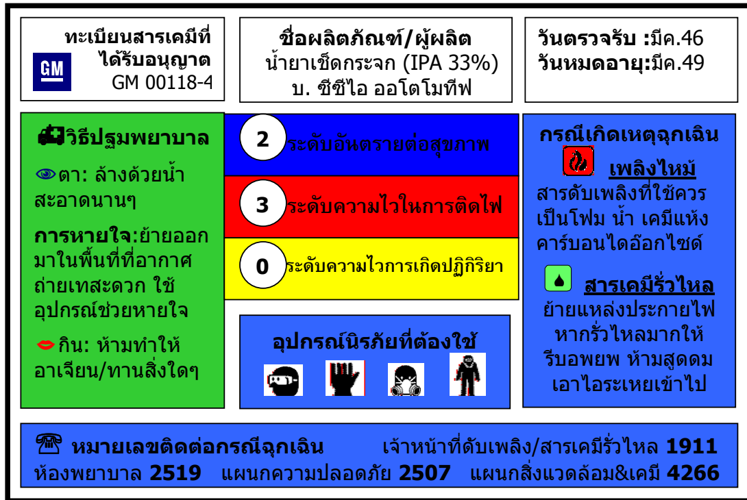
Figure 3-5: Designed label with Pictograms and Color codes but has no Signal word (SCY, MCY, LCY)
