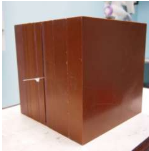
Figure 4.16 A 30×30×30 cm 3 cubic water phantom from slabs of solid water phantom.
