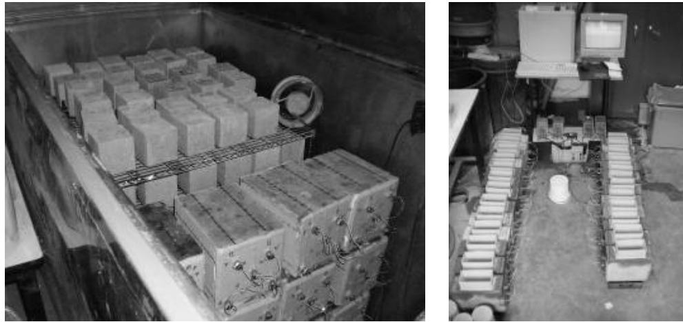
(a) Specimens in carbonation chamber (b) Ponding with chloride solution
