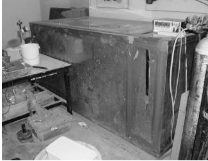
Figure 3.7 Carbonation chamber for carbonation depth test
