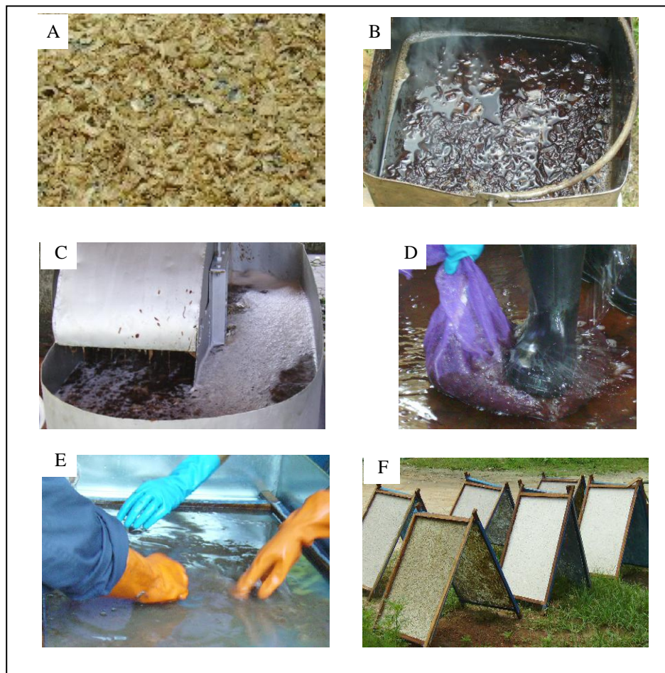
Figure 4.12 Process of banana paper production at Ron Phibun Sub-district (A) dried banana stem pieces (B) boiled stem pieces (C) beaten stem pieces (D) dewatered pulp (E) spread pulp on a frame (F) dried banana paper
