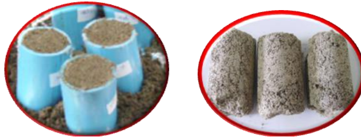
Figure 5.16 The 4 formulas of solidification/stabilization for arsenic
