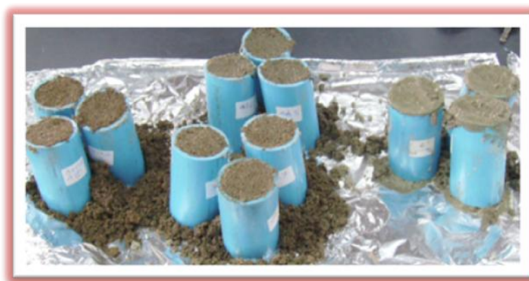
Figure 4.15 Solidification/stabilization of 4 formulas mixed with cement, ash, and sludge of arsenic contaminated wastes
