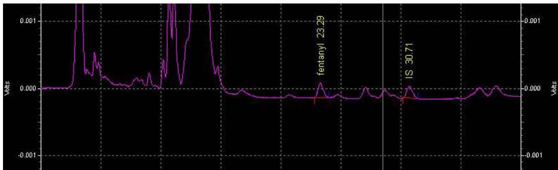
Figure 4.1 The chromatogram of reference standard (fentanyl and dimenhydrinate), blank plasma, zero blank plasma and QCM sample.
