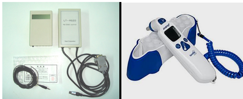
Figure 3.5 Thermistors for skin temperature [data logger (left)] and Tympanic Infrared Ear Thermometer (right)
