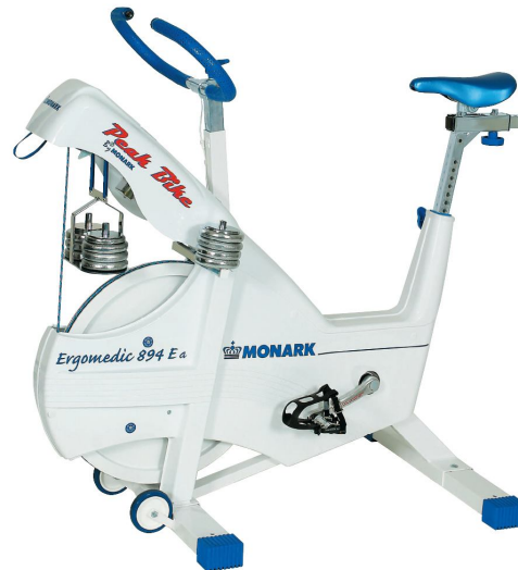
Figure 3.1 Standard Monark cycle ergometer for Wingate Anaerobic test.
