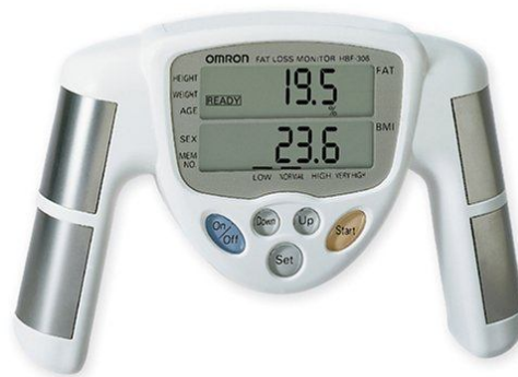
Figure 3.10 Body fat and composition device (Omron)
