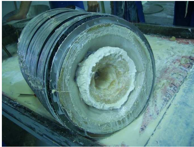
Figure 2-3 Centrifuged Residue from Centrifuged Process
