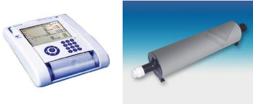
Figure 3.4 Pony FX desktop spirometer and Cosmed® syringe 3 liters
