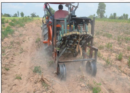
Fig.6 The back side of machine (Which removes gathering conveyer, cause be convenient to check the gripping after digging.)
