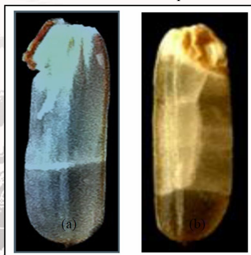
Figure 1 Crack feature on germinated rice surface a) Crack in cross-direction b) Crack in both cross and longitudinal directions
